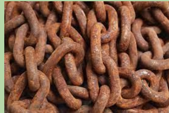
Rusting is the result of a chemical reaction between iron and oxygen.
