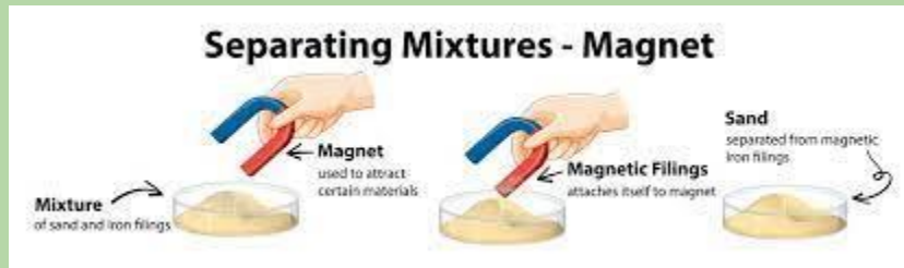
Using a magnet to separate iron filings from sand.
